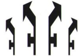
Arrows depicting that the first turn is prohibited but the second is permitted
