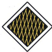
Box junction sign
