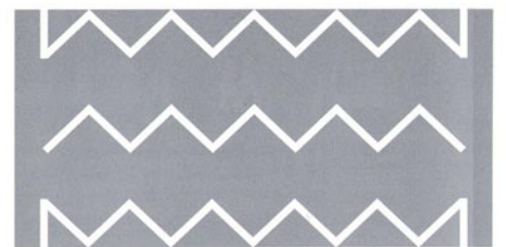
Zigzag lines: No parking, waiting or overtaking
