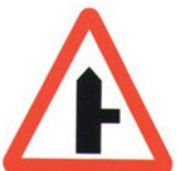
Junction on right ahead
