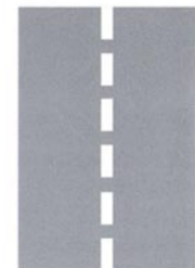
Lane dividers: overtaking is allowed
